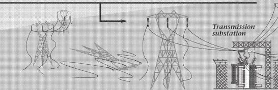
**Step 2.** A co-op may have several local distribution substations, each serving thousands of consumers. When a major outage occurs, the local distribution substations are checked first. A problem here could be caused by failure in the transmission system supplying the substation. If the problem can be corrected at the substation level, power may be restored to a large number of people.
